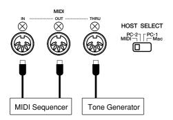
When you use the MIDI terminals, set the [HOST SELECT] switch to the MIDI position. The MIDI terminals will not transmit or receive data if this switch is set to any other position.
