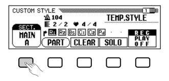
→ The **SECT.** function is highlighted, and each section is displayed in turn. The Clavinova plays the currently displayed section repeatedly.
