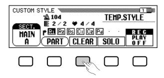
When recording a drum kit voice in part **R1** or **R2**, you can clear a single drum instrument from the part by pressing the key corresponding to the instrument to be cleared while holding down the C1 key on the keyboard. (The C1 key is labeled "CANCEL.") The metronome timing guide can also be cleared in this way.
