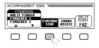
→ The **SYNCHRO STOP** function is highlighted, and the [SYNCHRO] lamp lights.
