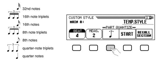
Once the required quantize size has been selected, press the **START** LCD button to quantize the current part. The part will begin to play using the new timing, and the **START** button will change to **UNDO**, allowing you to undo the quantize operation and return to the pre-quantized data if the results are not as you expected. You will not be able to **UNDO** once another button has been pressed.
