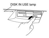
Never attempt to remove the disk or turn the power off during recording, reading and playing back. Doing so can damage the disk and possibly the disk drive.
