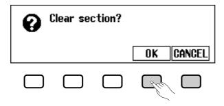
⇒ Press **0K** to clear the section, or **CANCEL** to abort. Once the style has been cleared, you can use the **MERS.** button, the data dial, or the [-] and [+] buttons to set the section length.
