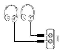
To use headphones, connect them to one of the [PHONES] jacks (standard 1/4" phone jacks) located below the left end of the keyboard. The Clavinova's built-in speaker system is automatically shut off when a pair of headphones are connected. Two people can enjoy listening to the Clavinova together by connecting two pairs of headphones to the two jacks.
