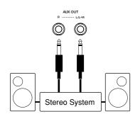
By connecting audio cables to the AUX OUT jacks as shown here, you can output the sound of the Clavinova to a stereo system, amplifier, mixing console, or recording equipment. Since the AUX OUT jacks provide output at a fixed level, you will need to use the controls on the connected equipment to adjust the overall volume of the sound from the Clavinova.
