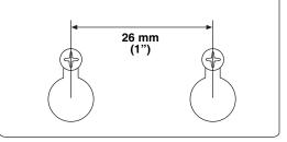
Fasten screws into a firm wall or wall support as shown in the figure below, and hang the holes on the protruding screws.
