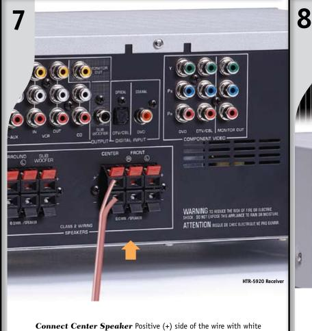
stripe attaches to (+) terminal. Negative (-) side attaches to (-) terminal.
