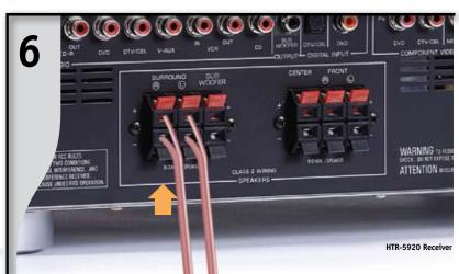
**CAUTION** Receiver must not be plugged in while connecting speakers. Connect Surround Speakers Positive (+) side of the wire with white stripe attaches to (+) terminal. Negative (-) side attaches to (-) terminal.
