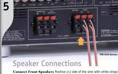
attaches to (+) terminal. Negative (-) side attaches to (-) terminal.
