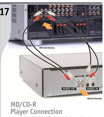
**Connect MD/CD-R Recorder (optional)** Connect RCA audio cables (not included) to "MD/CD-R" terminals on receiver as shown.
