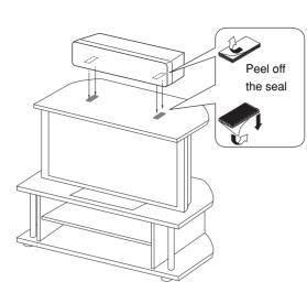
When placing the speaker on top of the TV rack, etc., attach the provided fasteners at two points on the bottom of the speaker and on the top of the TV.
