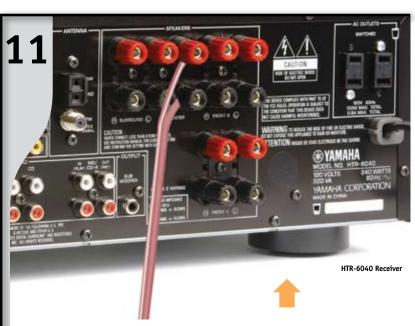
Connect Center Speaker Positive (+) side of the wire with white stripe attaches to (+) terminal. Negative (-) side attaches to (-) terminal.
