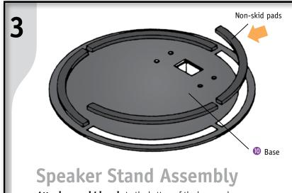
Attach non-skid pads to the bottom of the base as shown. Repeat steps for each base.
