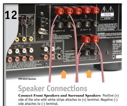
**CAUTION** Receiver must not be plugged in while connecting speakers.
