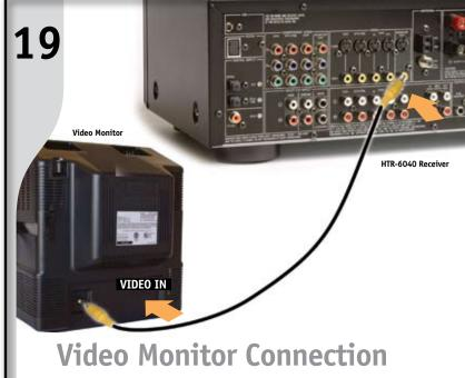
**Connect a Video Monitor (optional)** Connect an RCA video cable (not included) to receiver Monitor OUT from your video monitor as shown.
