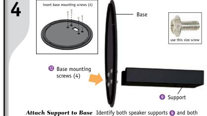
bases 10 and attach support to base using the four short screws 12 as shown. Do not over-tighten the screws. Doing so may damage the screws or assembly. Repeat steps for each base.
