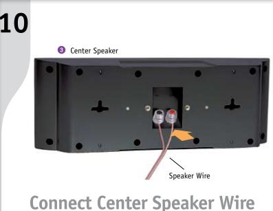
Connect Center Speaker Wire as shown. The positive (+) side of the wire with the white stripe attaches to the red terminal. The negative (-) side attaches to the black terminal. Place all speakers in desired location as shown in Step 2, Room Layout.
