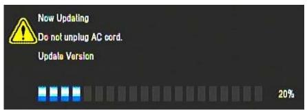
While update is in progress, **DO NOT** interrupt the power or press any buttons.
