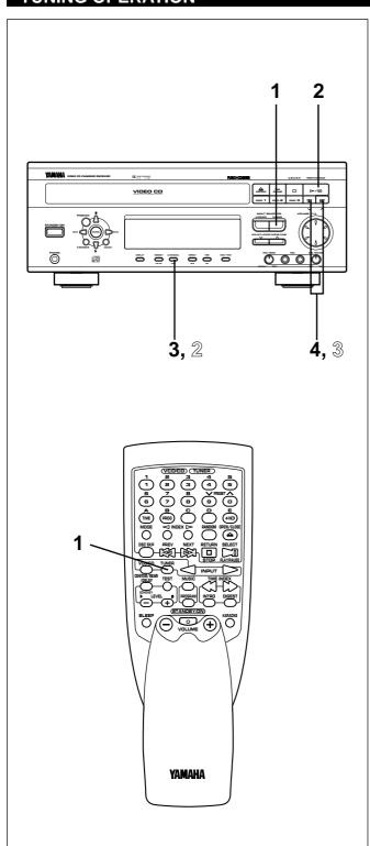
Normally, if station signals are strong and there is no interference, quick automatic-search tuning (Automatic tuning) is possible. However, if signals of the station you want to select are weak, you must tune to it manually (Manual tuning).
