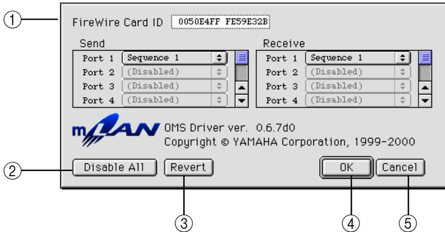
In this dialog box, you can use the pop-up menus in the “Send” and “Receive” columns to specify which mLAN MIDI sequences (that are transmitted and received by the computer) are assigned to which port.
