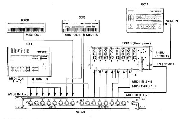
\* NOTE: Module 1 should always be switched to "Common" and the other modules to "Individual".
