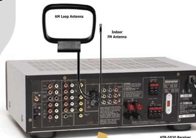
**Connect Antennas to Receiver** Locate AM loop antenna and indoor FM antenna. Keeping receiver unplugged, connect as shown. For more information about obtaining clear reception and grounding, see your Owner's Manual.
