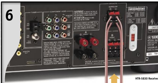
**Connect Surround Speakers** Positive (+) side of the wire with white stripe attaches to (+) terminal. Negative (-) side attaches to (-) terminal.
