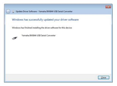
Click [Close] to close the window, and check that "Yamaha IMX644 USB Serial Converter" has been added to the "Universal Serial Bus controllers" item in the Device Manager window.
