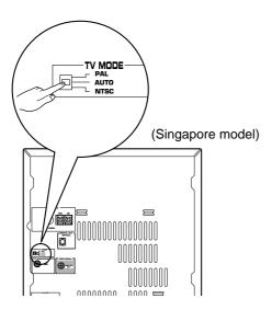
This system is designed for use with the NTSC and PAL television formats. Set this switch to the position for the format your TV monitor employs.
