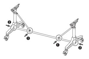
4. Lock the casters by pressing the stoppers on the left and right casters.
