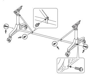
After making sure that each joint is connected, securely tighten
