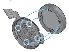
The L and R orientation of the earpads does not matter. The earpad that has stitching on the side goes down.
