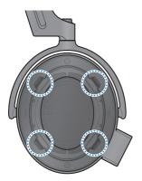
2 If the earpad comes off of one of the fastening points, pull on each of the fastening points in order to take the earpad off.
