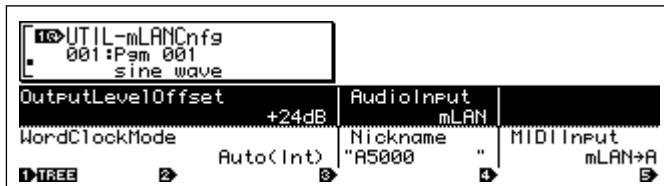
**(NOTE)** Output Level Offset, Word Clock Mode, and Nickname settings are saved in the mLAN8E. They cannot be saved on disk.
