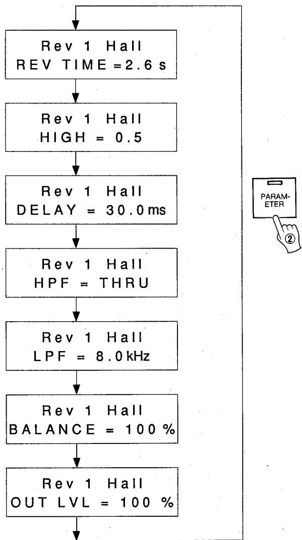
Note that the first parameter in the list is returned to if the PARAMETER button is pressed after the last parameter (OUT LVL in this example) has been called.
