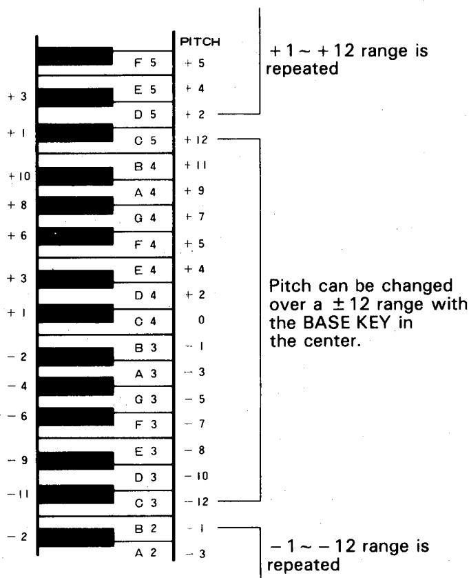
PITCH CHANGE B makes it possible to produce two independently pitch-shifted output notes in addition to the direct signal, so you can actually create three-part harmonies with a single input note. Both pitch-shifted notes appear at the center of the stereo sound field (i.e. they are output equally to the L and R OUTPUT jacks).
