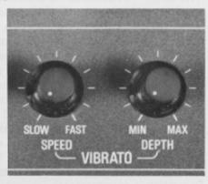
Note: The rate of "wah-wah" included in tones of "funny" and "wah guitar" as a preset part of the voice, can be altered using the vibrato controls. Place the vibrato lever (3) to "control" position, set the vibrato depth control (section 6) to the minimum (counterclockwise) position. You can now adjust the vibrato speed control to obtain the desired rate of wah without introducing a vibrato effect.
