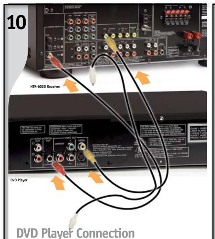
Connect DVD Player (optional) Top: Connect RCA audio/video cables 8 to receiver: Yellow to "DVD," Red to "Digital Input DVD Coaxial" as shown, and leave White unplugged. Bottom: Connect audio/video cables to DVD player from receiver: Yellow to "Video", Red to "Coaxial", and leave White unplugged.
