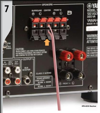
Connect Center Speaker Positive (+) side of the wire with white stripe attaches to (+) terminal. Negative (-) side attaches to (-) terminal.
