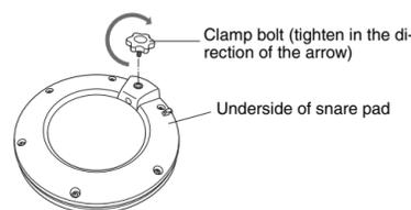
2. Push the snare pad onto the rack's snare holder. Ensure that the snare holder's rod is fully inserted into the snare pad's mounting hole, and then tighten the clamp bolt to secure the pad in place.
