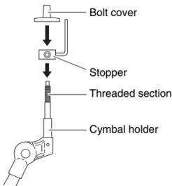
5. With the stopper making full contact with the bottom surface of the bolt cover as shown below, tighten the stopper's key bolt using the tuning key.
