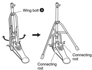
5. As shown on the right, loosen the hi-hat clutch's wing bolt **b** and remove the hi-hat clutch.
