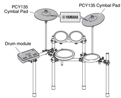
A cymbal pad's built-in sensor is located close to the Yamaha logo found on the top surface. In order to achieve the best performance from your pad, position it such that the area around the logo can be easily struck. (See the figure above.)
