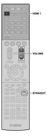
Press HDMI 1 to select "HDMI 1" as the input source.
